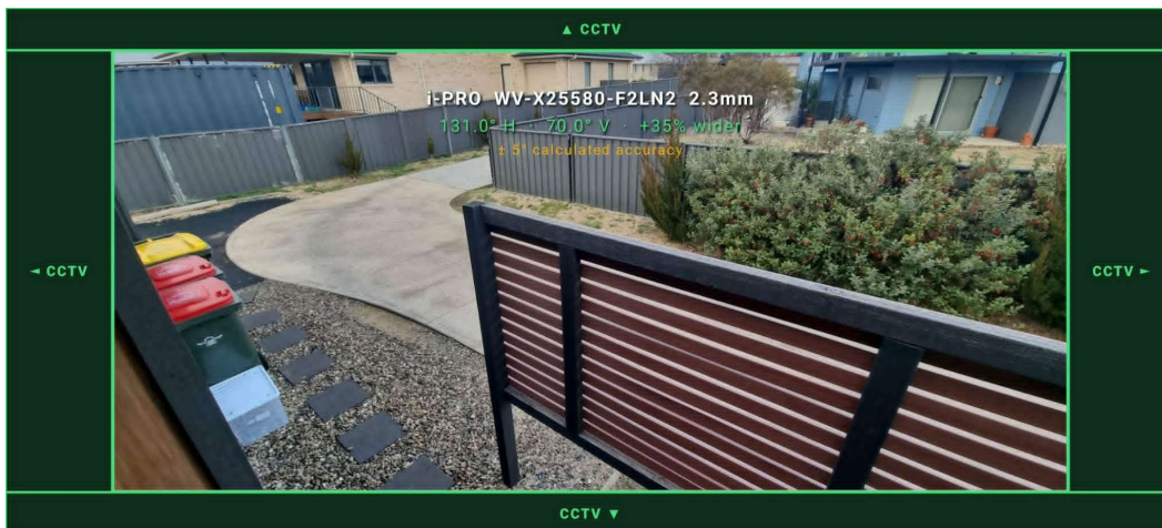
Wider case: the i-PRO WV-X25580-F2LN2 at 2.3mm covers 131° horizontally. The green frame marks CCTV coverage extending beyond the phone image on all four sides.
